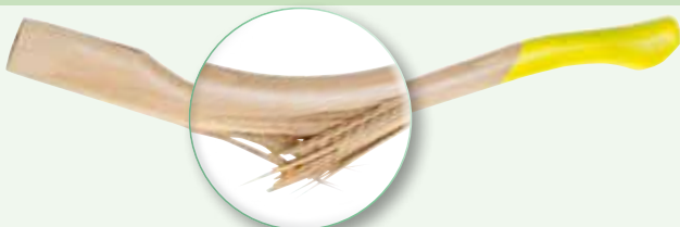
Break point on a hickory handle
